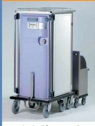
The tray with food from the meal plating belt is placed into the trolley (capacity 16, 20, 24, 28 & 30 level). Once loaded the trolley is docked with a Stand-Fresh compressor unit for a 20 minute boost period whereby the hot shelves are thermalised and the cold section chilled at each level during the same cycle. The trolley is then un-docked and transported to ward level with temperatures
