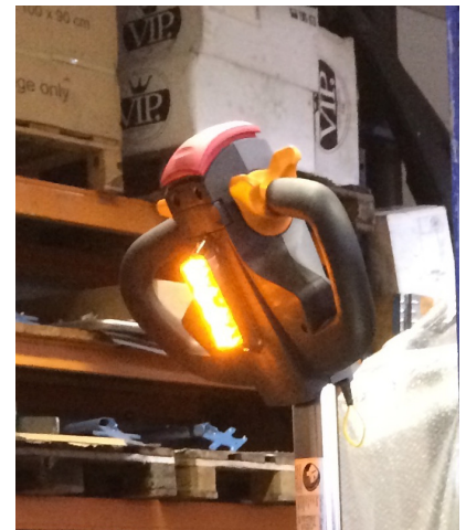
Flashing Warning Light P/N: 3601515ass Dimensions: 120 x 40 x 30 mm
